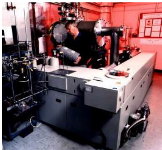
Figure 6. The Bruker Optics IFS 120HR Fourier Transform Spectrometer at Rutherford Appleton Laboratory
