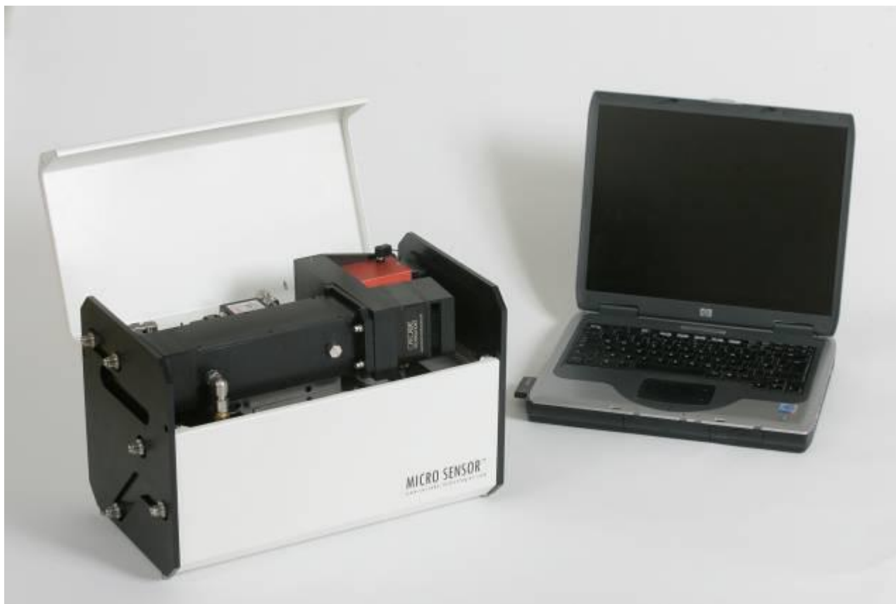
Figure 7. Example of Prototype Laboratory Demonstrator Gas Sensor developed at Cascade Technologies .Cascades' proprietary control electronics and software exploit the key advantages provided by its patented intra pulse technique.
